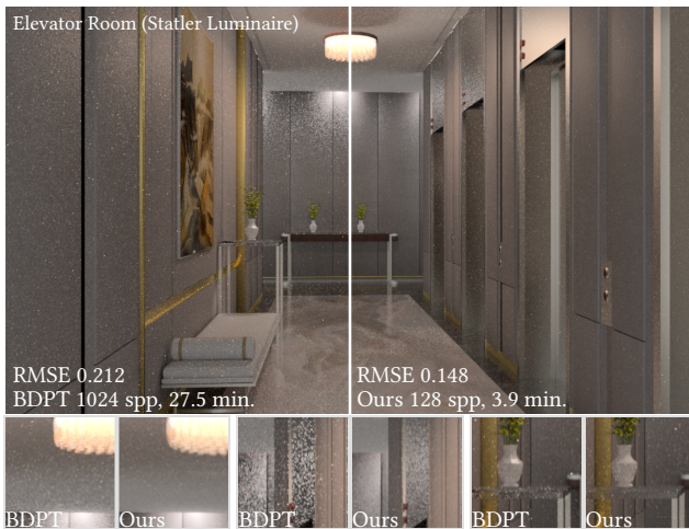
Fig. 10. Comparison with BDPT which takes significantly more samples to converge since many paths fail to connect with paths from the hidden emitters at the top of the glass tubes. Our approach can query the luminaire directly without having to evaluate costly paths resulting in relatively less noise with fewer samples and a 7× speed up in render time.
