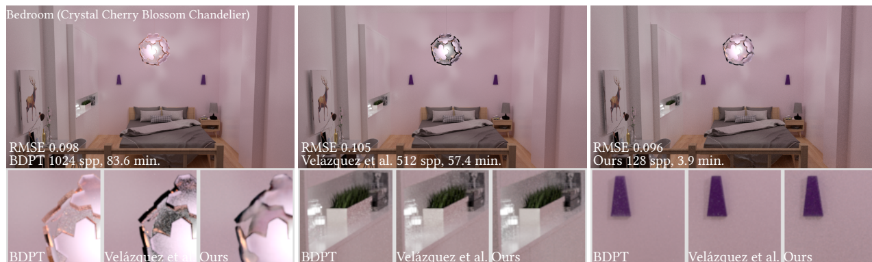
Fig. 12. The glass petals of the luminaire obfuscate light paths and create high frequency shadows on the walls our method preserves. Moreover, we capture the direct appearance more accurately than the state-of-the-art method from Velázquez et al. and demonstrate a speedup of nearly 22× relative to BDPT.
