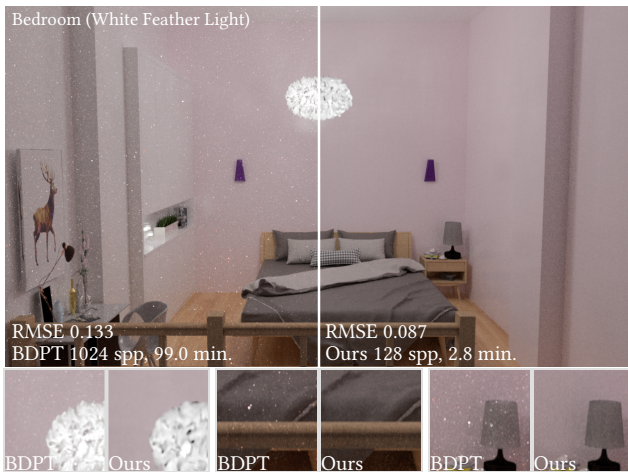
Fig. 17. Non-transparent feathers on a glass ellipsoid shell cover two emitters resulting in extremely complex light transport. BDPT still contains residual noise relative to our approach despite its 36× longer render time.
