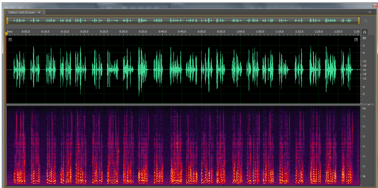
Figure 30. Test 2 – BF Effect on Raw Echo, Time Domain and Spectrogram (BF Enabled; AER Disabled)
