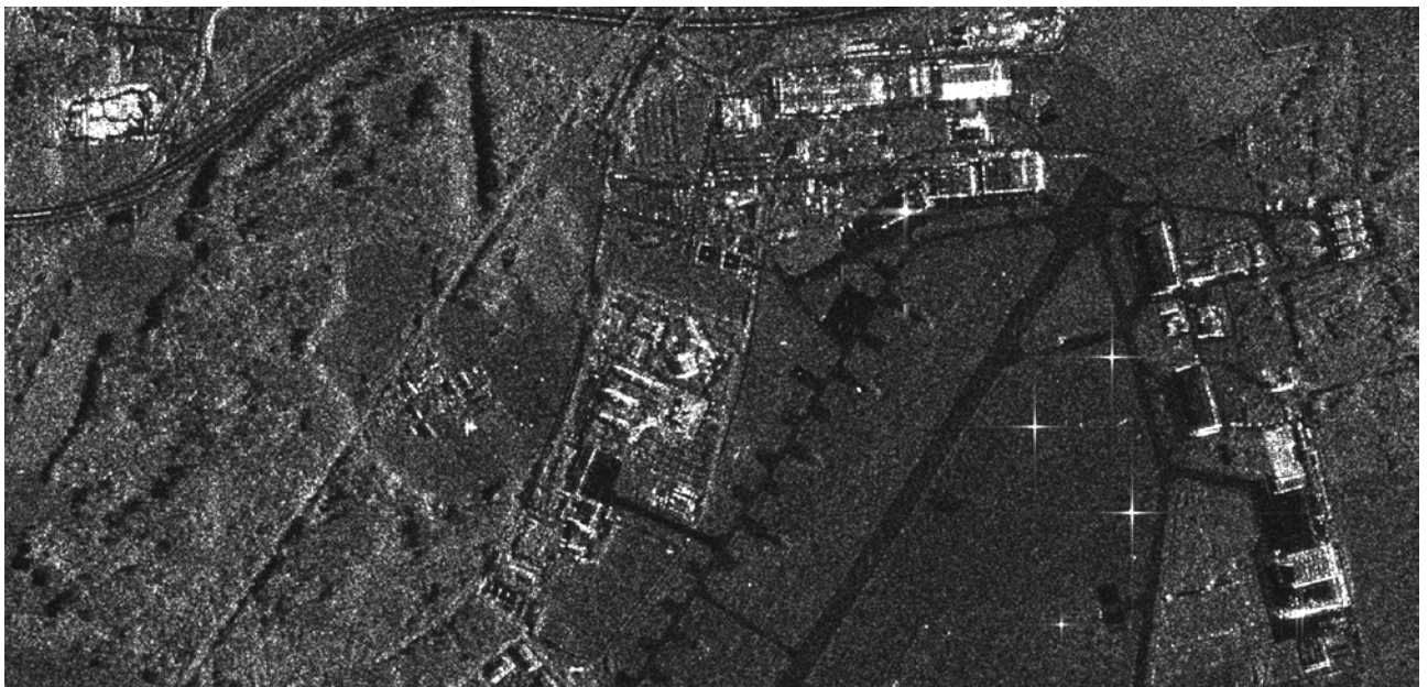
Fig. 3-1: Example for a spatially enhanced stripmap product with 1.2 looks and approx. 3.2 meter resolution of the Oberpfaffenhofen calibration site. The extent is 2.9km x 1.4km (pixel spacing: 1.25m)
