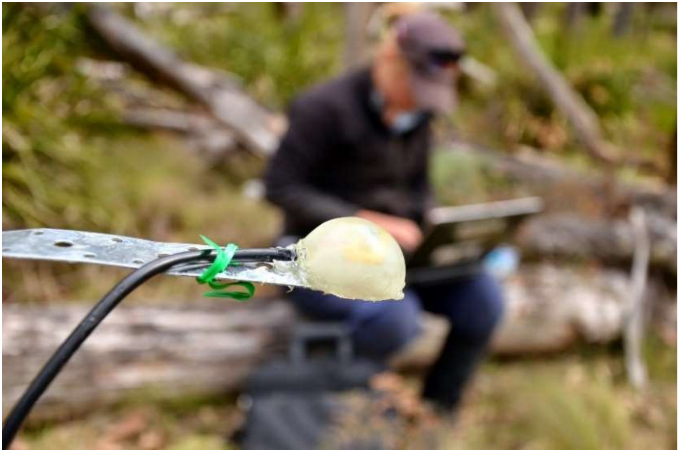
Fig. 2 Photoresistor encapsulated in a clear epoxy dome and mounted in the field on a metal bracket
