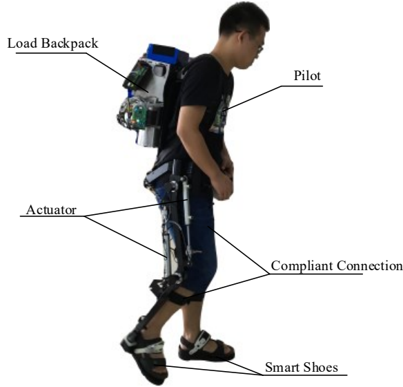
Figure C1 HUALEX with the pilot. The pilot and HUALEX are connected with compliant connections. The hip joints and knee joints are driven with bi-directional linear hydraulic cylinders. The smart shoes are used for detecting gait phases.
