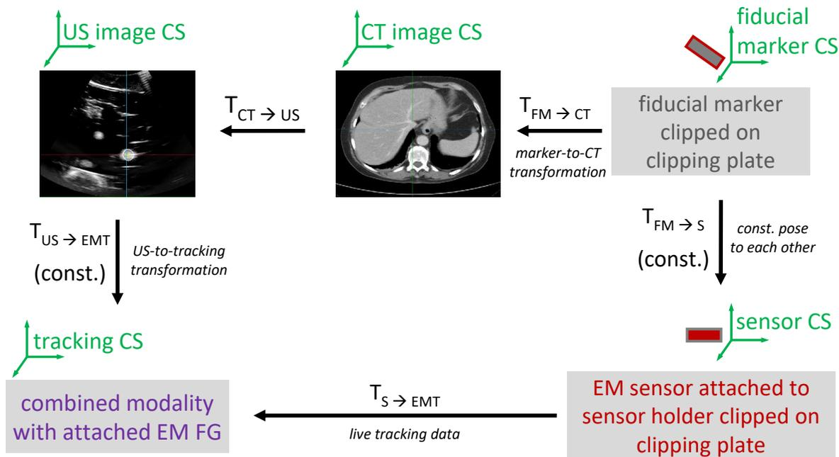
Figure 2: Transformation chain required for registering the CT data to the US image space. Abbreviations: CS = coordinate system; CT = computed tomography; EM = electromagnetic; EMT = electromagnetic tracking; FG = field generator; FM = fiducial marker; S = sensor; US = ultrasound.
