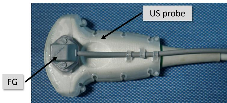
Figure 1: Combined modality used in the abdominal phantom study.
