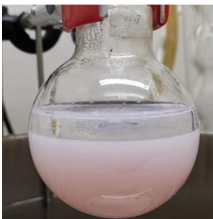
Figure S1 The photo picture of the reactor for the synthesis of the Au@MSN by the biphasic stratification approach. The heterogeneous oil-water stratification reaction system shown in the figure contains the tetraethyl orthosilicate (TEOS) solution as a silica source in hydrophobic organic solvent as the upper oil phase, while the lower pink phase is the solution of the products, which contains monodisperse gold suspensions as core, cetyltrimethylammonium chloride (CTAC) as a template, and triethanolamine (TEA) as a catalyst.
