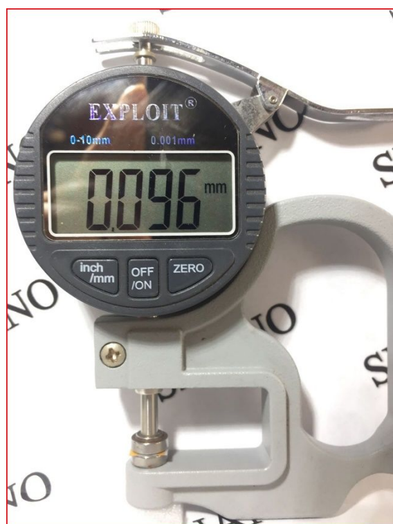
Fig.S11 Photograph of gas sensor thickness measurement.
