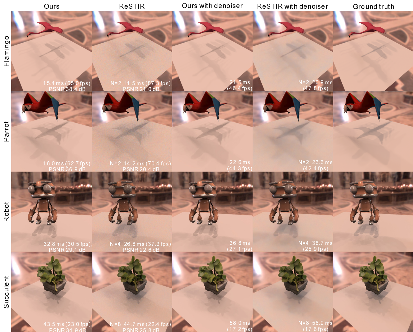
Fig. 3 The direct illumination rendering images of our algorithm and ReSTIR [1] given simple 3D models. For each model, with the similar per frame processing time, the rendering images of ReSTIR in the second column have noticeable pepper noise, while the rendering images of our algorithm in the first column practically have no noise and capture the subtle shadow transitions to an extent equivalent to the ground truth in the last column. In terms of PSNR, our algorithm provides a visual quality improvement around 10 dB w.r.t. ReSTIR. Applying the AI denoiser [3] removes the noise, but the subtle shadow transitions are also blurred in the denoised images of ReSTIR in the fourth column.
