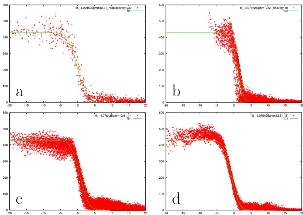
Figure S7: Plots of the density variation across rounded portions of the crystal (a), and across planar boundaries of the crystal (b-d). Fits to error functions (solid lines) were used to obtain the apparent thickness of the density boundary. The units of the horizontal axis are in pixels of 14nm.
