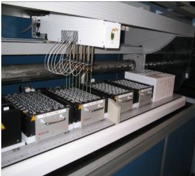
Figure 12 - Customized Tecan robots are used to pipette solutions onto the slides at precisely programmed intervals, allowing the majority of the ISH procedure to be performed in an automated fashion.
