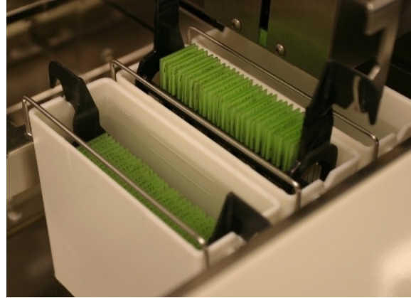
Figure 10 - Leica Autostainer XL's are used for the fixation and dehydration tasks. Acetylation is performed manually.
