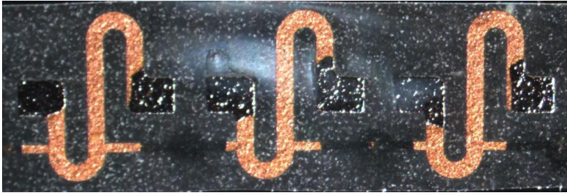
Supplementary Figure S7 Selective electroplating. (a) A picture of selectively electroplated circuit. (b) For selective electroplating, the meandering lines were partially marked with manicure.
