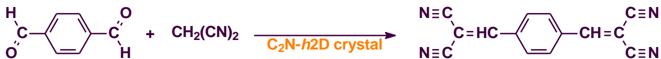
Supplementary Figure 19 | Schematic presentation of Knoevenagel condensation reaction of terephthalaldehyde and malononitrile in the presence of the C 2 N-h 2 D crystal as a reaction catalyst.
