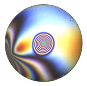
Endfacet of the laser-machined fiber used in the experiment. Picture taken with a home-buit white-light interferometric microscope. The fiber endfacet is mirror coated with a commercial IBS coating (R=99.9976%,  $T=L=12\,ppm$ ) from ATF, Boulder.
