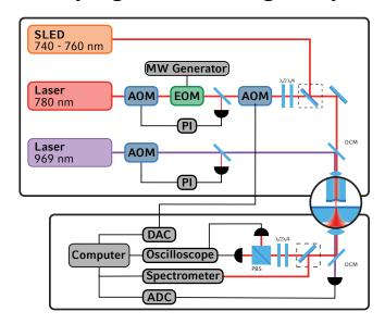
**Probe laser** The cavity is probed by a grating stabilized external cavity diode laser (TOPTICA DLpro) at a wavelength of 780 nm. The power of the laser ist stabilized to a relative noise level of  $10^{-4}$  by a feedback loop consisting of an AOM, a PI controller and a photodiode.
