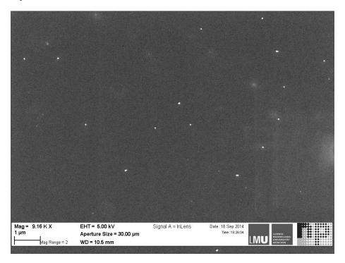
Scanning electron microscope image of mirror with gold nanospheres used in the experiments.
