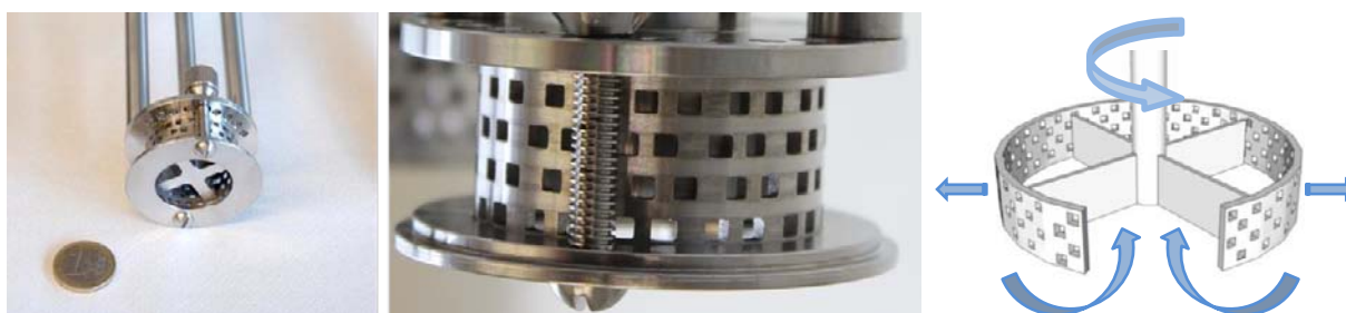
Figure S1.1: Close up view of the D=32\ \text{mm} rotor/stator used in this work and (right) a schematic illustrating the operation of the rotor stator. The top arrow indicates the direction of rotation while the other arrows illustrate the direction of liquid (and associated solids) flow.
