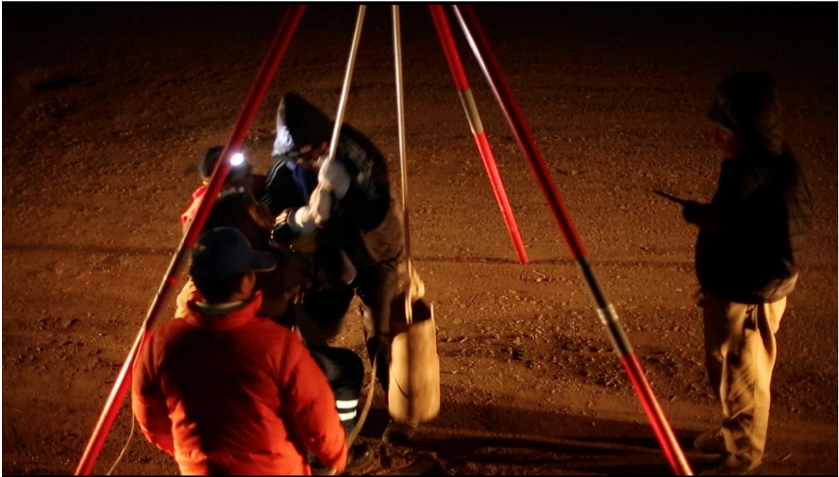
Supplementary Figure 11 | Estimation of the P wave velocities in the Maca landslide. Picture of the source system. An 80-kg mass was pulled up to approximately 2 m high using a tripod and a pulley and dropped onto a metallic plate. Data were acquired at night to diminish the impact of wind and anthropogenic noise (mainly coming from a road attracting considerable tourist traffic) on the signal recorded.
