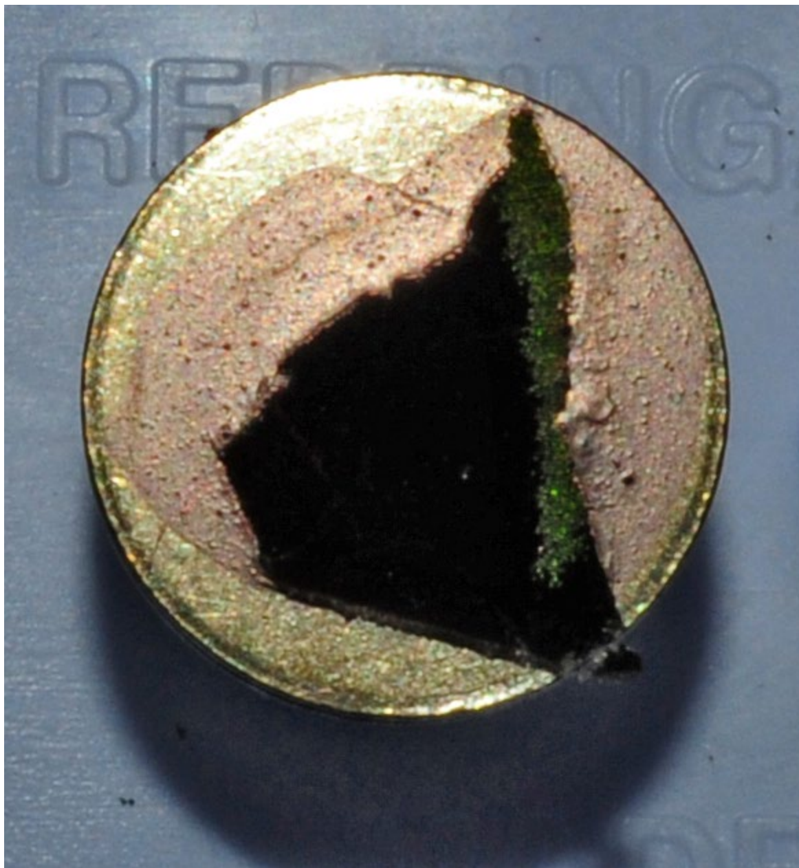
Supplementary Figure 3. Piece of butterfly wing sputter coated with gold. Ultra-black butterfly wings are still black when coated with gold, indicating that there is a structural component to the absorption.
