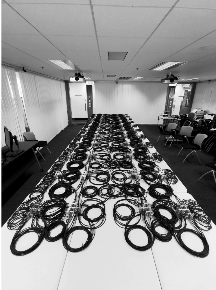
Supplementary Figure 13. Transmission line network constructed for charges \pm q_{14} , where around 880 coaxial cables are used.
