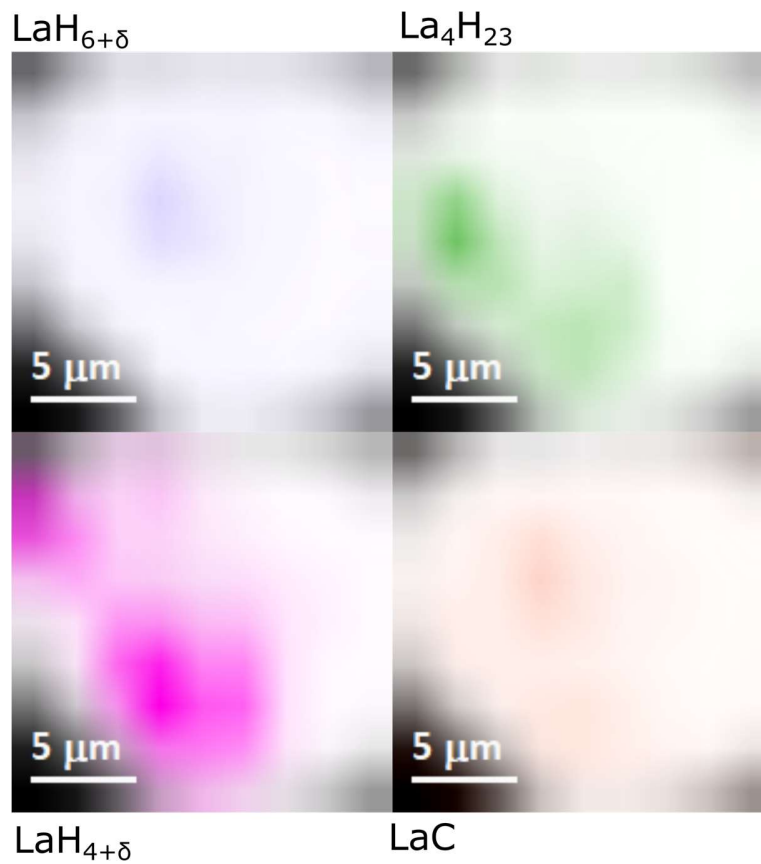
Supplementary Figure 3: Sample X-ray diffraction map at 150 GPa, collected as 9x9 images with 2 \mu\text{m} steps. For each phase, an X-ray diffraction line not significantly overlapping with that of another phase was selected. For \text{LaH}_{6+\delta} , \text{La}_4\text{H}_{23} , \text{LaH}_{4+\delta} and \text{LaC} , the 16.40 , 6.82 , 6.51 , and 13.77^\circ 2\theta peaks ( \lambda = 0.29521 \text{ \AA} ) were selected, respectively. Each panel shows the XRD map with one phase visible, with the color's intensity being proportional to the intensity of its X-ray diffraction line. To allow comparison between images, all intensities were normalized to the most intense peak out of any phases ( i.e. \text{LaH}_{4+\delta} ). Due to preferred orientation, selected peaks chosen at high and low 2\theta values, these maps can solely be used for a qualitative interpretation.
