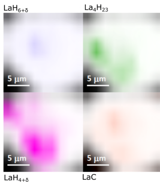
Figure S3: Sample X-ray diffraction map at 150 GPa, collected as 9x9 images with 2 \mu\text{m} steps. For each phase, an X-ray diffraction line not significantly overlapping with that of another phase was selected. For \text{LaH}_{6+\delta} , \text{La}_4\text{H}_{23} , \text{LaH}_{4+\delta} and \text{LaC} , the 16.40, 6.82, 6.51, and 13.77° 2\theta peaks ( \lambda = 0.29521 \text{ \AA} ) were selected, respectively. Each panel shows the XRD map with one phase visible, with the color's intensity being proportional to the intensity of its X-ray diffraction line. To allow comparison between images, all intensities were normalized to the most intense peak out of any phases ( i.e. \text{LaH}_{4+\delta} ). Due to preferred orientation, selected peaks chosen at high and low 2\theta values, these maps can solely be used for a qualitative interpretation.
