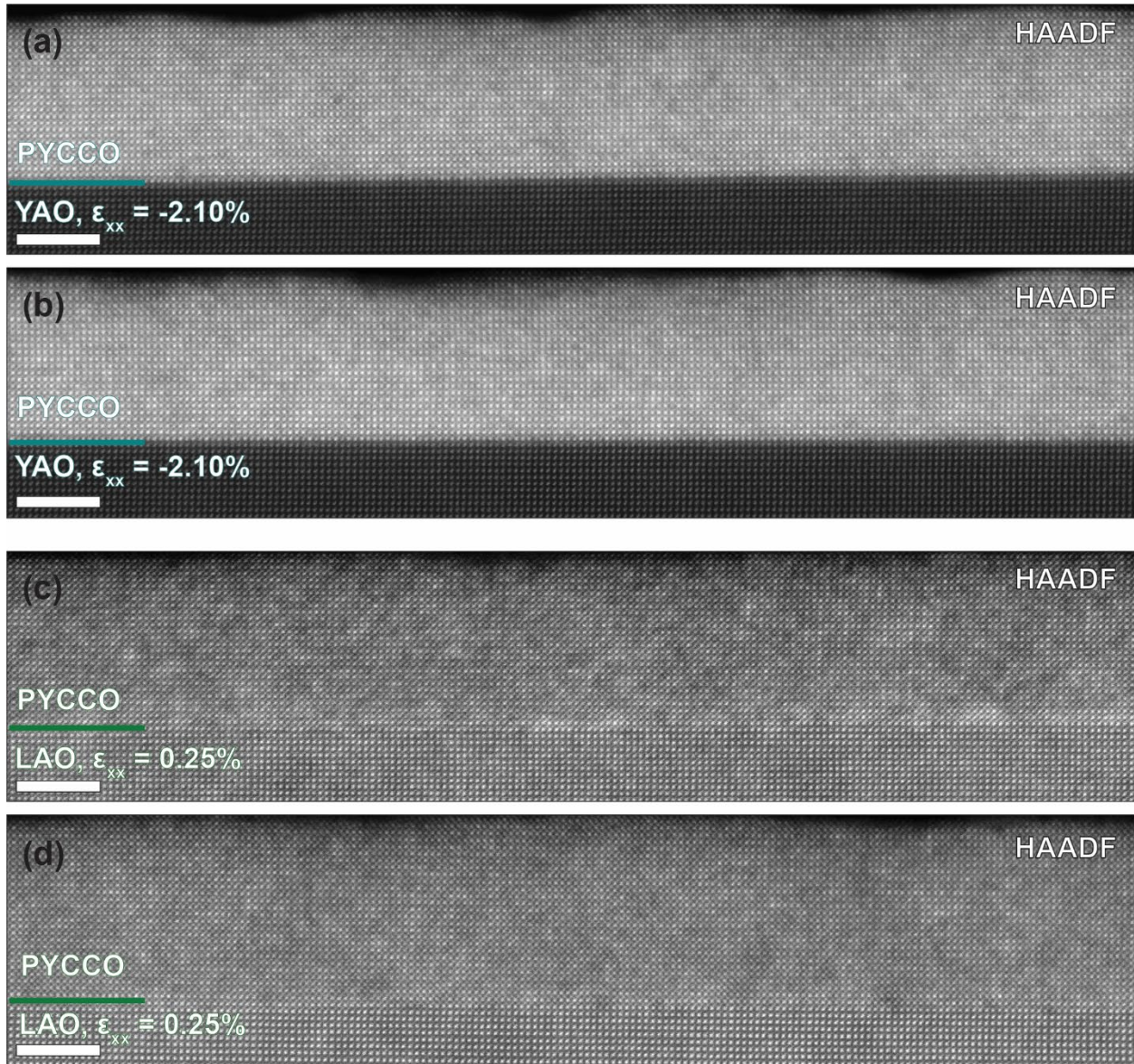
Figure S2: Additional electron microscopy characterization. Atomic-resolution high-angle annular-dark-field scanning transmission electron microscopy (HAADF-STEM) images of \sim 26 -unit-cell-thick (\text{Pr}_{0.85}\text{Y}_{0.15})_{0.7}\text{Ca}_{0.3}\text{CoO}_{3-\delta} (PYCCO) films on YAO(101) ( \epsilon_{xx} = -2.10\% ) and LAO(001) ( \epsilon_{xx} = 0.25\% ) substrates. (a,b) HAADF-STEM images of different regions of a PYCCO film on YAO. (c,d) HAADF-STEM images of different regions of a PYCCO film on LAO. The scale bars are 5 nm, and the horizontal lines mark the interfaces. As noted in the main text, the local HAADF intensity variations due to doping fluctuations are evident throughout the images. No superstructure due to, e.g. , O vacancy order, is observed in any case.
