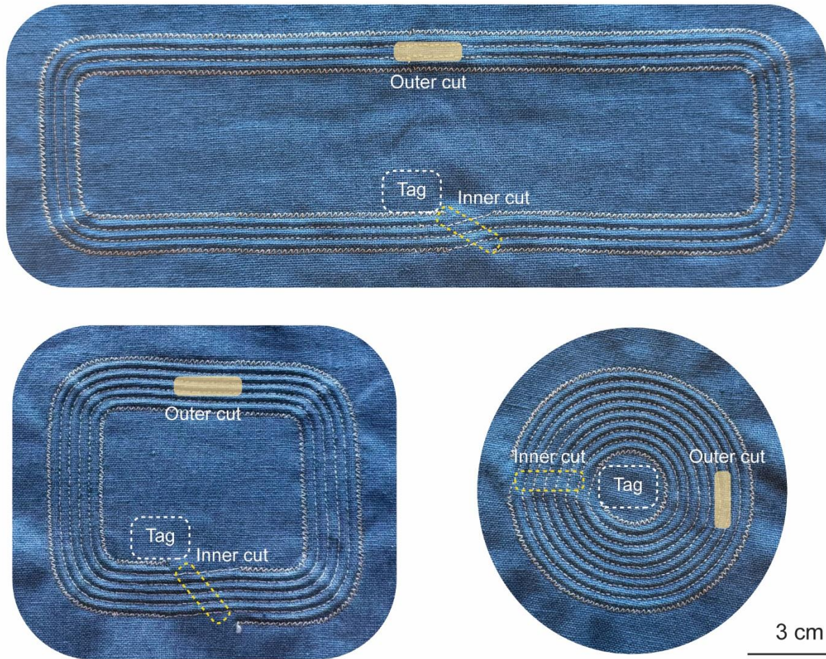
Supplementary Figure 24. Alternative textile NFC antenna designs by leveraging the programmable digital embroidery patterns. a Antenna with the same size as the metamaterial, potentially integrated into the BAN to serve as both a tag (receiver) and transmission relay simultaneously. b Antenna with larger size for increased operation range. c A round antenna with more turns and higher filling ratio to eliminate the use of tuning capacitor.
