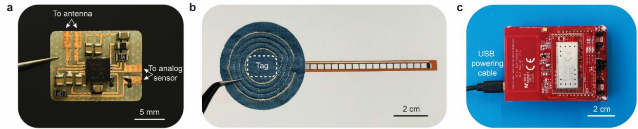
Supplementary Figure 15. NFC tag and reader. a Picture of the fabricated 16 mm × 12 mm circuit board (through PCB milling) of the NFC transponder. b NFC tag integrated with a commercial strain sensor and a coaxially-shielded NFC antenna embedded in textile through digital embroidery. c Picture of the adopted commercial NFC reader with a 4 cm × 2 cm reader antenna, powered by a USB cable through a laptop.
