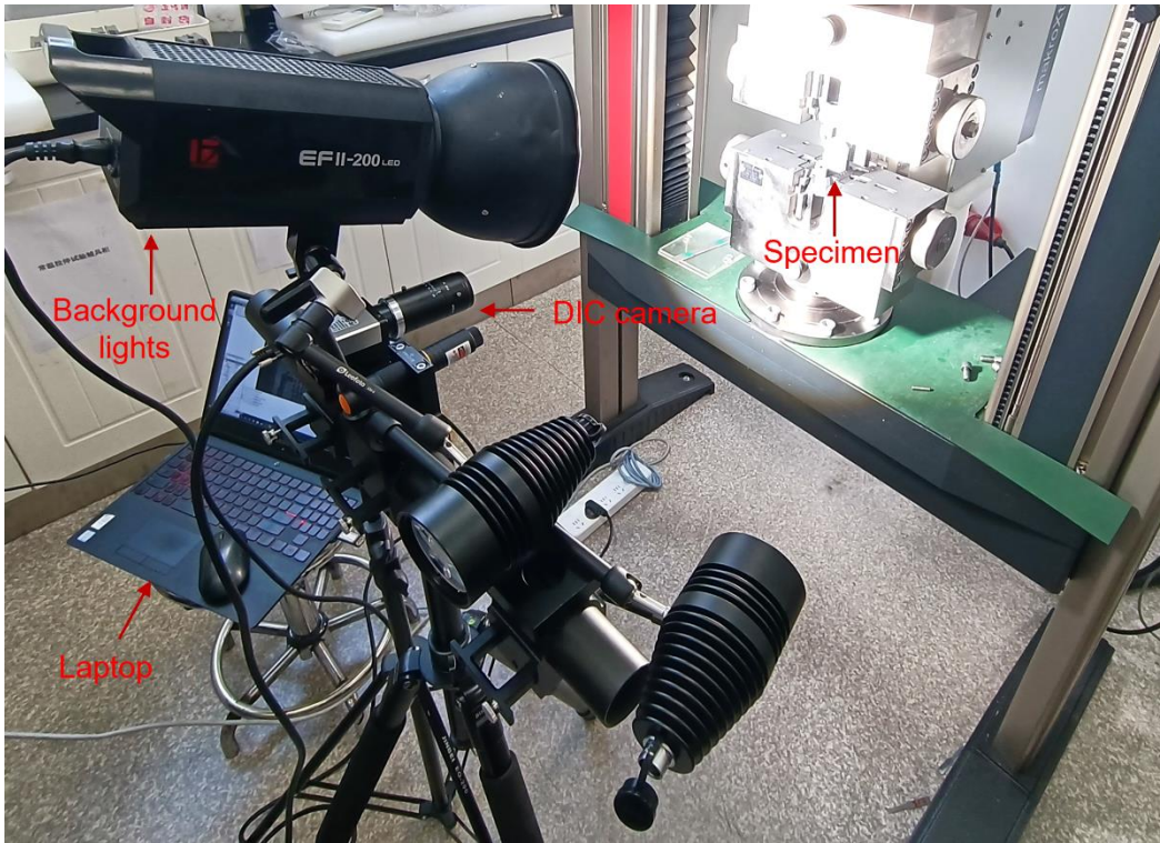
Supplementary Fig. 18. Experimental configuration of the digital image correlation (DIC) analysis.
