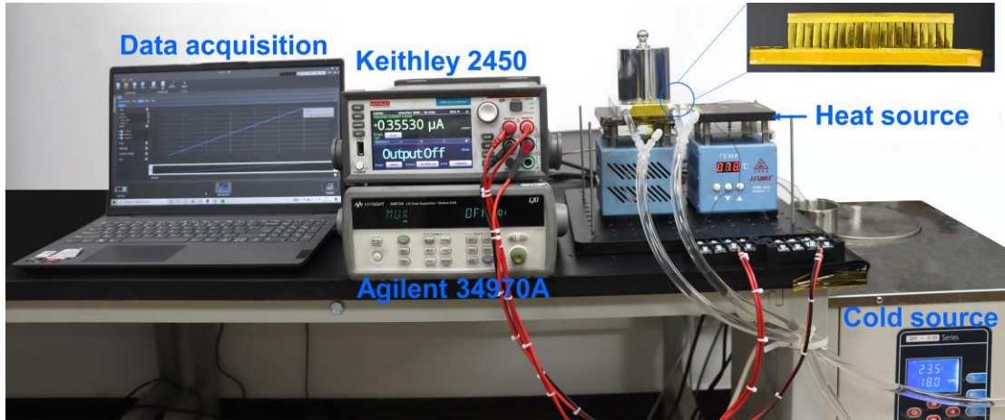
Fig.44| The FTEG performance test platform: the voltage and current was obtained under different temperature difference of the FTEG cold/hot sides.
