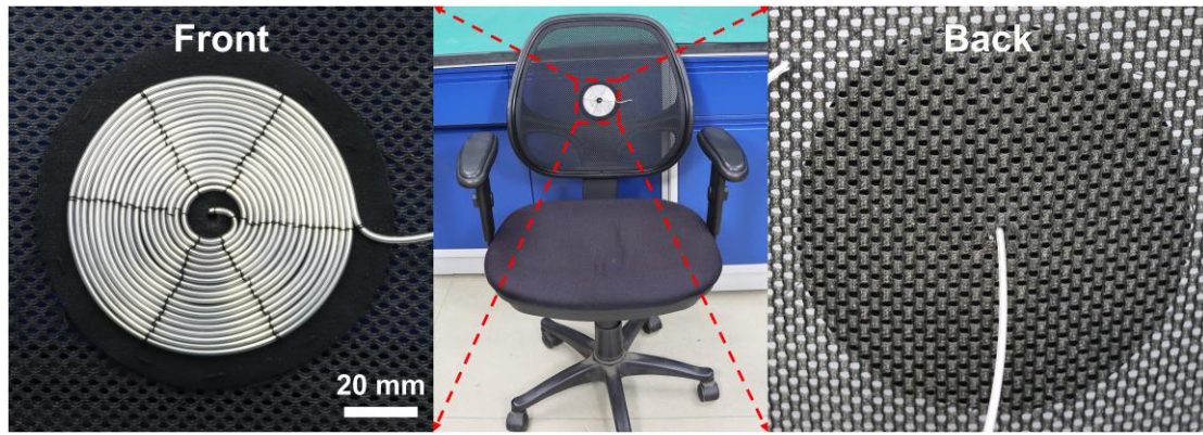
Fig.35| The spiral-shaped transmission coil, winding with a flexible tube filled with the room-temperature liquid metal of GaInSn, is woven into the back of the chair.
