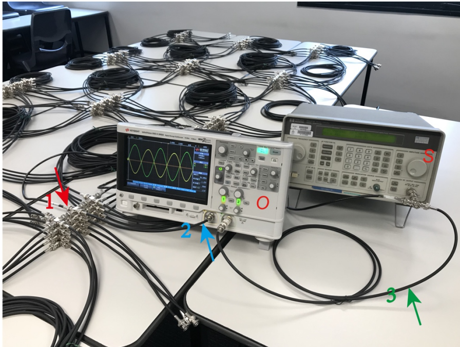
Figure S25 | Setups for the experimental measurements. ‘S’ indicates the signal generator (Keysight 8647A Synthesized Signal Generator), and ‘O’ is the oscilloscope (Keysight DSOX2002A Oscilloscope). The AC frequency signal from the signal generator is input to the nodes of one meta-atom by cable 1 (red arrow). The short cable 2 (cyan arrow) is used to measure the voltage at each node without breaking the original system. The cable 3 (green arrow) is used to provide a reference signal for the phase measurement.
