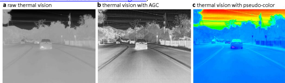
Fig.11 State-of-the-art approaches to improve visual contrast. To visualize more details, (b) AGC maps raw pixel values from grayscale to grayscale, while (c) pseudo-coloring maps raw pixel values from grayscale to RGB.
