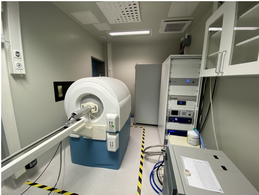
Figure S1: Preclinical 7 Tesla MR Scanner (MRS*DRYMAG, MR solutions, Guildford, UK) used for MRI image acquisition.
