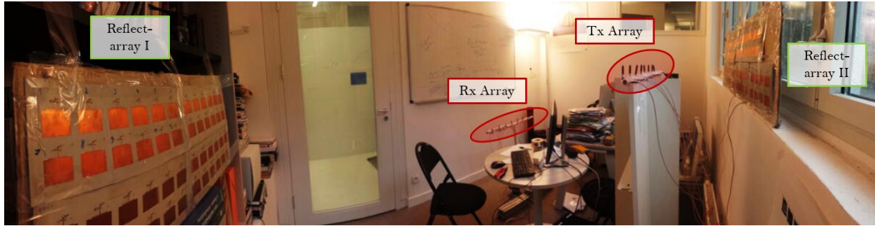
Supplementary Figure 6 | Photographic image of the office room setup. Two antenna arrays are placed in a heavily furnished office of irregular geometry. The two parts of the metasurface reflect-array are also identified in the image.
