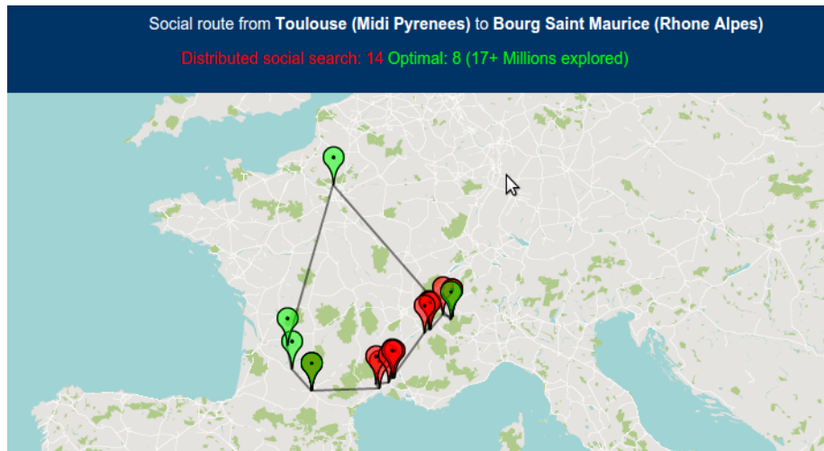
Fig. S7: Snapshot of the app we developed for visualize our results. The red route is the result of distributed ran-com-deg while the green one displays the optimal route. In this example, the distributed route needs 14 steps to reach the destination city, while the optimal route uses 8. However, the distributed algorithm explores only 123 nodes, while more than 17 million nodes are checked for finding an optimal route. Figure created using using map tiles from openstreetmap.org (OpenStreetMap contributors 6 , licensed under Creative Commons BY-SA 2.0 licence. To view a copy of this license, visit creativecommons.org/licenses/by-sa/2.0 ).
