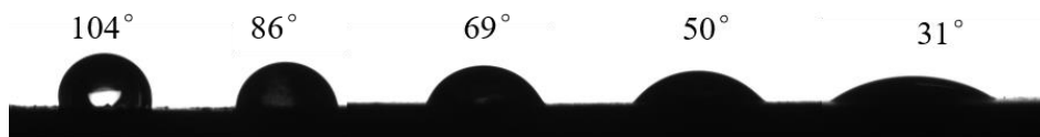
Figure S5. The water contact angle along the wettability gradient surface. The graphite plate is treated at a constant current of 0.5 A and the volume flow is 1 L/h. Clearly, wettability gradient is formed after gradient oxidation treatment. The scale bar is 1mm.
