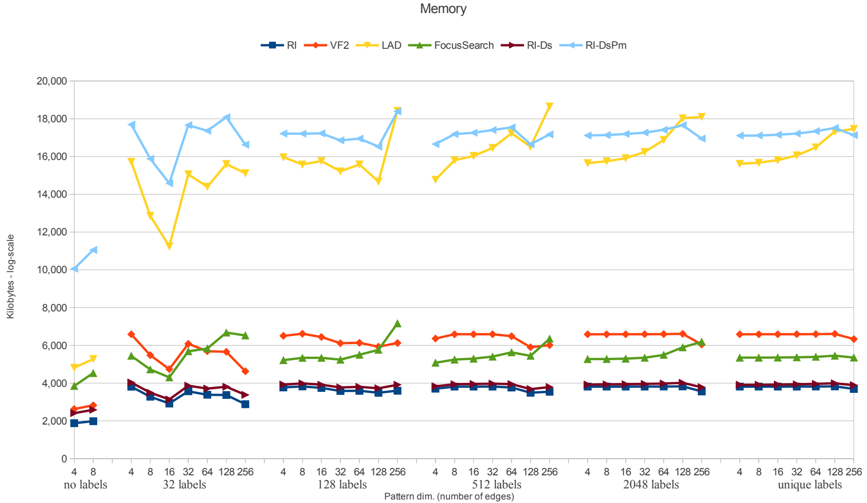
Figure 28: Averages of memory requirements for the Graemlin datasets. Networks are randomly uniformly labeled with 32, 64, 128, 512, 2048 and all different labels. Results are grouped by number of labels in the dataset and pattern dimension (number of edges). The chart measures the peaks of memory usage during the execution of the algorithms. The large number of nodes in the target graphs does not make the memory usage in LAD explode in contrast to the amount of memory requirement to store compatibility maps and domains. However, thanks to the bit vector domain representation, FocusSearch can maintain a reasonably low memory usage. RI outperforms all other systems.
