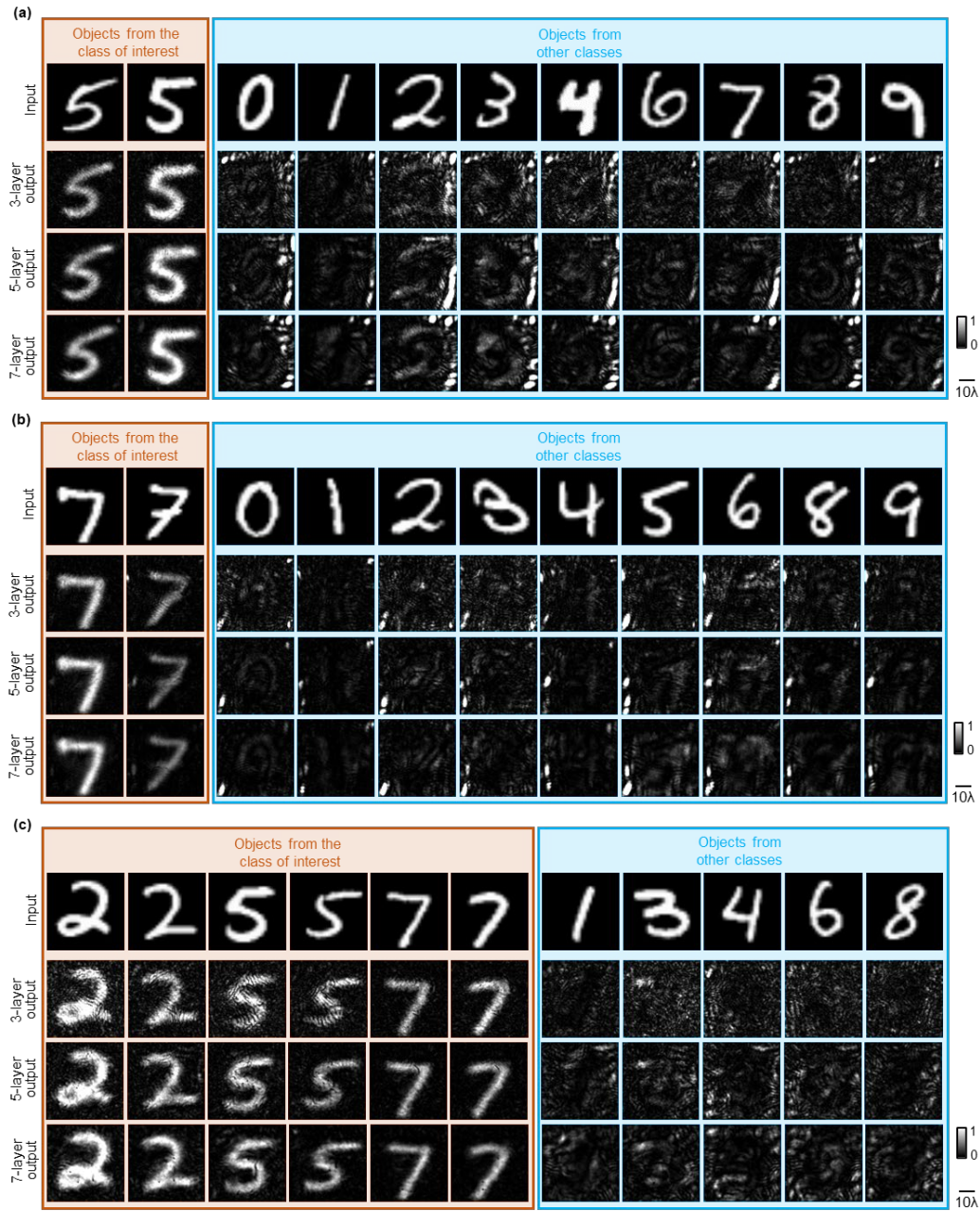
Figure S1. Blind testing results of diffractive camera designs that selectively image different data classes. (a) Blind testing results of a three-layer, a five-layer, and a seven-layer diffractive camera design when the target class of interest was chosen as the handwritten digit ‘5’. (b) Blind testing results of a three-layer, a five-layer, and a seven-layer diffractive camera design when the target class of interest was chosen as the handwritten digit ‘7’. (c) Blind testing results of a three-layer, a five-layer, and a seven-layer diffractive camera design when the target classes of interest were chosen as digits ‘2’, ‘5’, and ‘7’ - altogether. The output images at each row were adjusted using the same constant for visualization.
