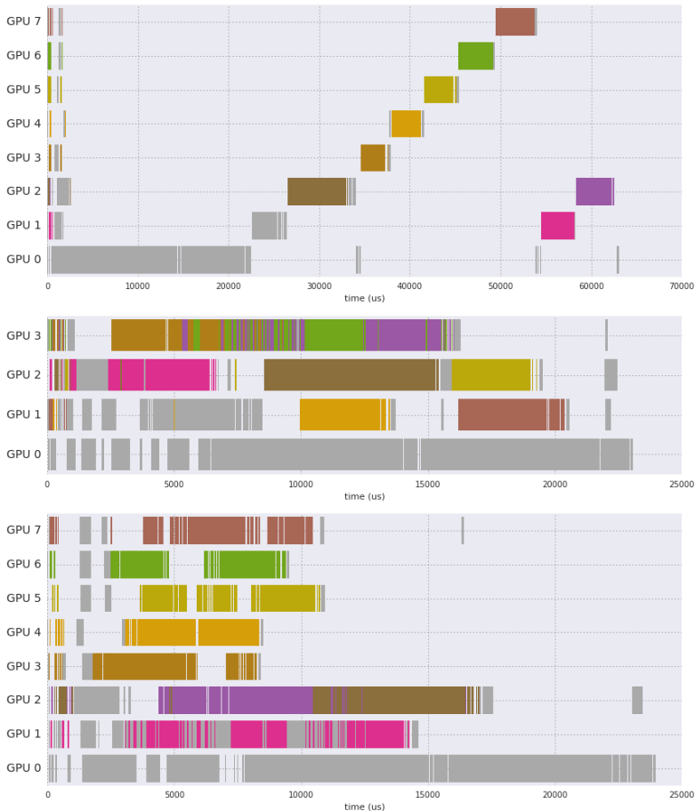
Fig. 1. Timeline for GPU usage for a sequential Par-Inception model on 8 GPUs at the top, a semi-parallel Par-Inception model using 4 GPUs in the middle, and a fully parallel model on 8 GPUs at the bottom. Each inception block is represented with a different color. Operations outside of inception blocks are colored in grey. Note that the timescale is different in the first picture compared to the two following ones.
