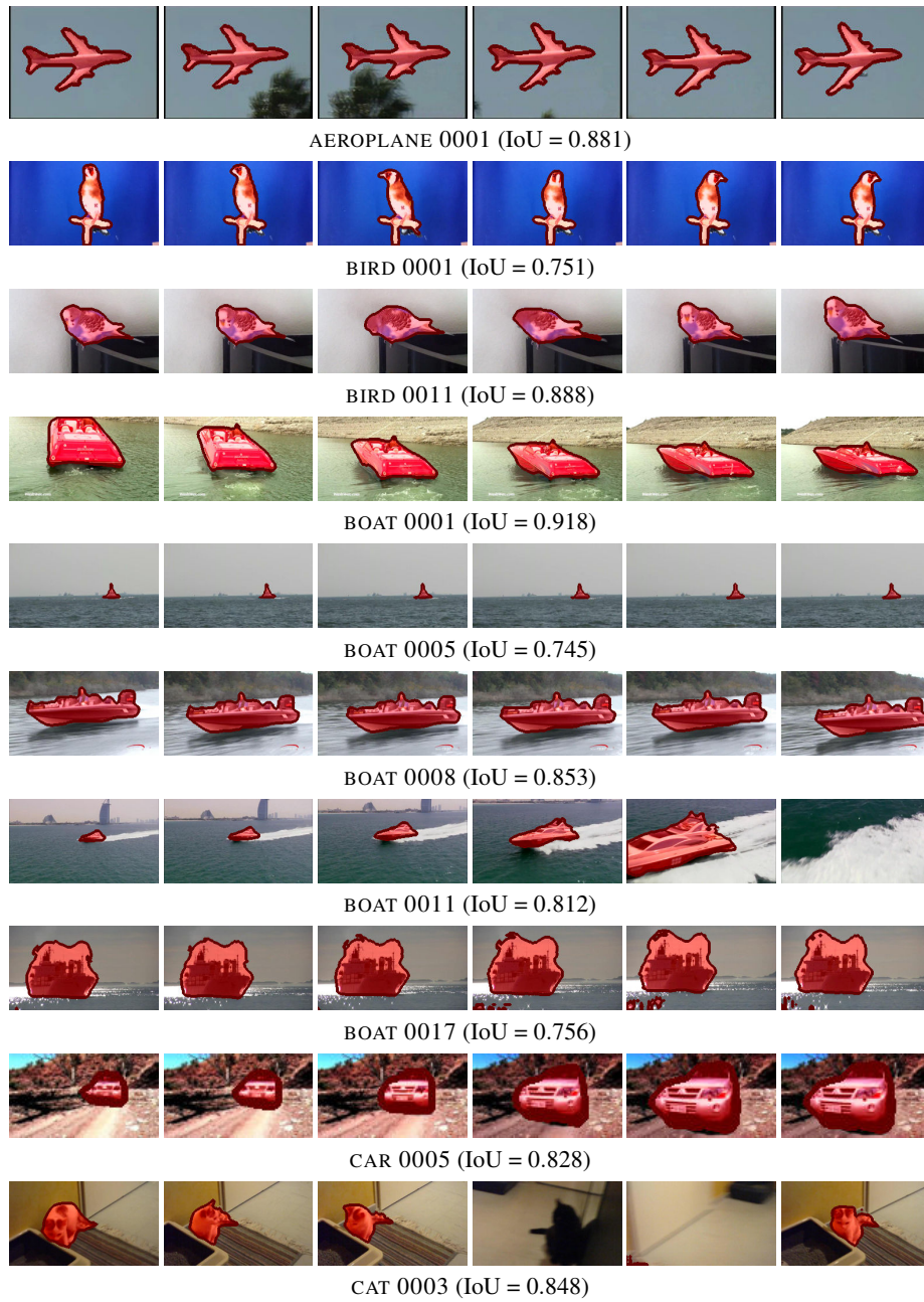
Fig. 3: Results of our approach on the YouTube-Objects dataset. The six frames are uniformly sampled from each video.
