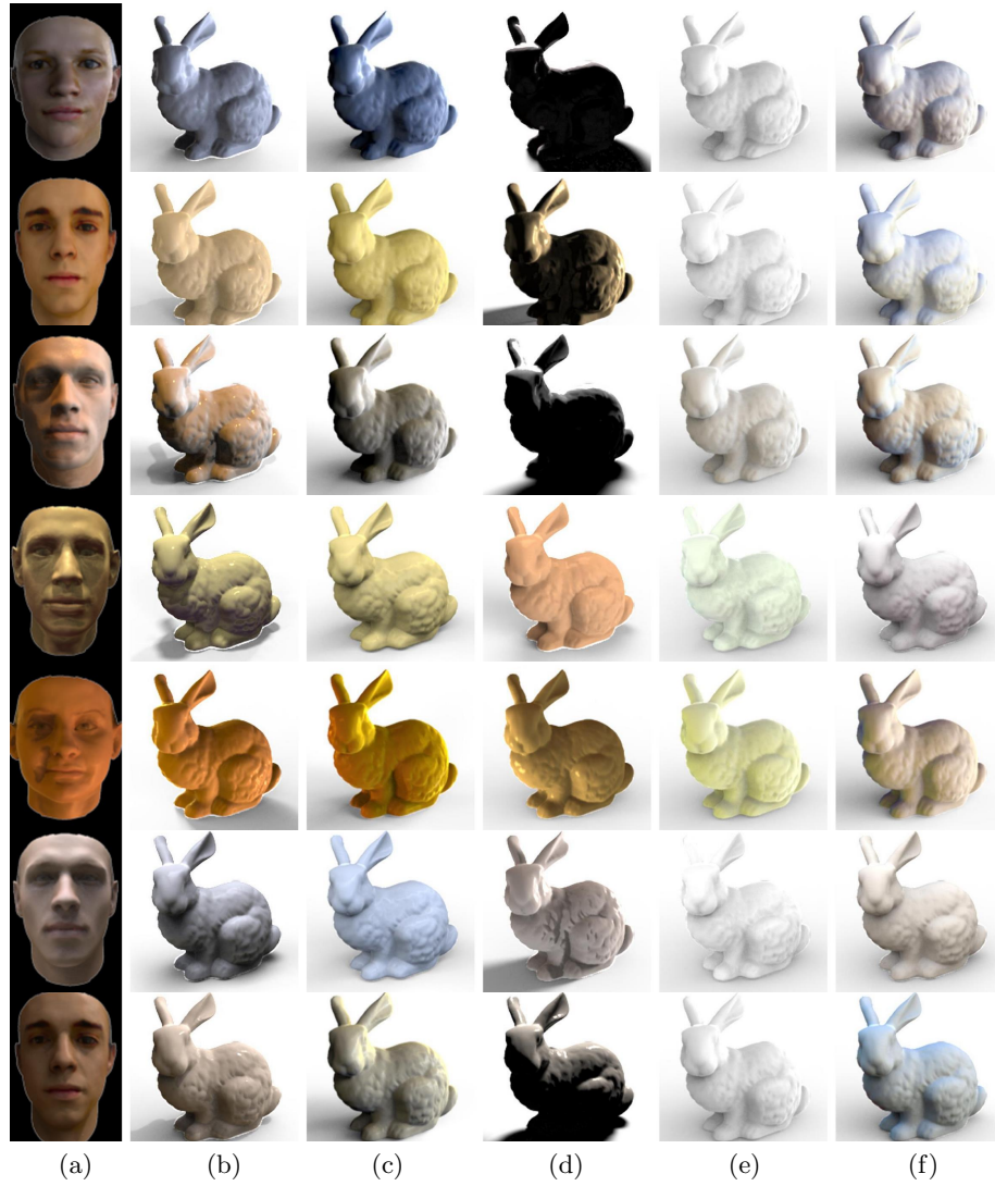
Fig. 23. Comparisons of glossy Stanford bunny relit by estimated indoor illuminations. (a) Input photo. (b) Bunnies under ground truth environment maps. (c-f) Bunnies relit by environment maps estimated by (c) our method, (d) [1], (e) [7] and (f) [4].
