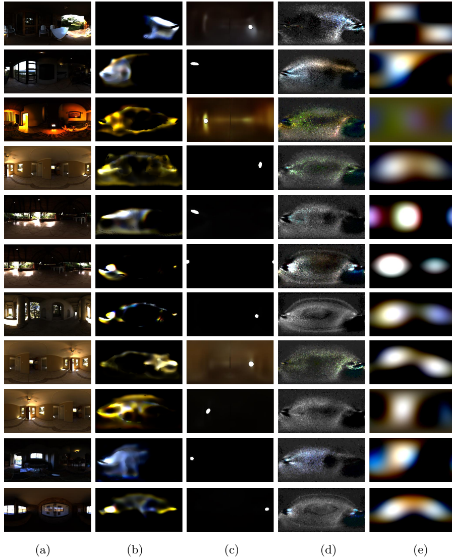
Fig. 24. Comparisons of selected indoor data used in quantitative evaluation of illumination estimation. (a) Ground truth indoor environment maps, (b-e) indoor environment maps estimated by (b) our method, (c) [1], (d) [7] and (e) [4]. Total intensities of all environment maps are normalized to be the same.
