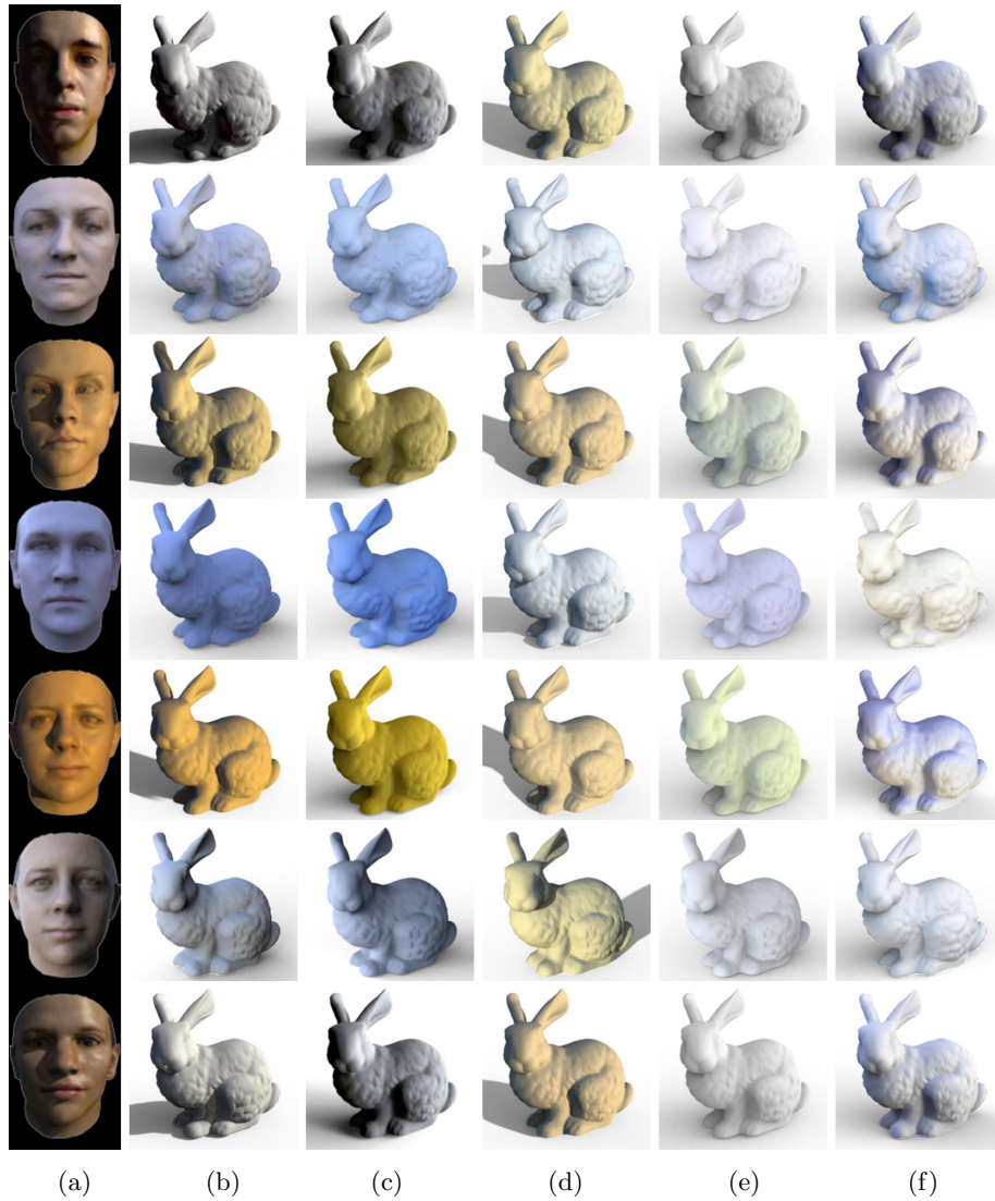
Fig. 17. Comparisons of diffuse Stanford bunny relit by estimated outdoor illuminations. (a) Input photo. (b) Bunnies under ground truth environment maps. (c-f) Bunnies relit by environment maps estimated by (c) our method, (d) [3], (e) [7] and (f) [4].
