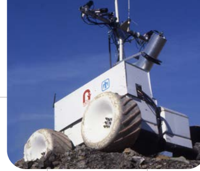
RATLER - PROTOTYPE ROVER BUILT TO DEMONSTRATE TECHNOLOGIES THAT COULD ENABLE ROBOTIC LUNAR MISSIONS.
