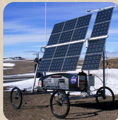
HYPERION: SUN-SYNCH - A SOLAR POWERED ROVER THAT PROVED THE CONCEPT OF SUN-SYNCHRONOUS NAVIGATION IN THE CANADIAN HIGH ARCTIC.
