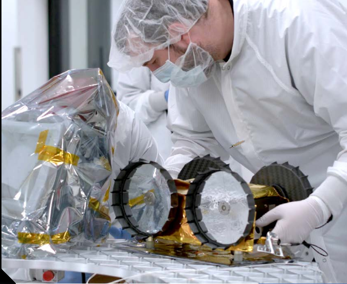
Tim Angert, the RI Machine Shop Manager, integrating the Iris rover on the lander deck.
