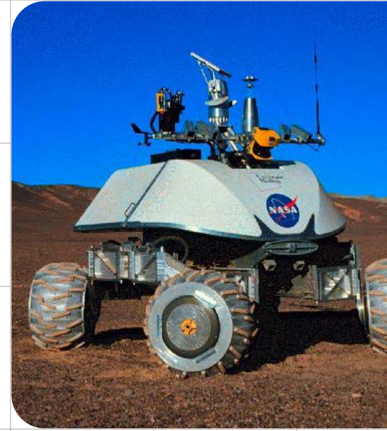
NOMAD - BUILT FOR AUTONOMOUS EXPLORATION OF PLANET-LIKE DESERTS; PIONEERED SPHERICAL VISION AND LONG-RANGE NAVIGATION.
