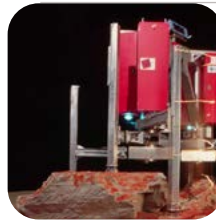
AMBLER - A WALKING ROBOT DEVELOPED AS A TESTBED FOR RESEARCH IN WALKING ROBOTS OPERATING IN RUGGED TERRAIN.
