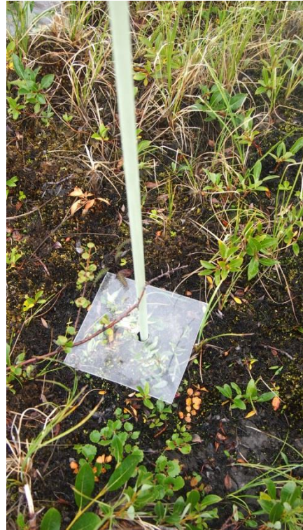
Figure 2. a) Metal pipe, anchored in permafrost; b) fiberglass rod, anchored in permafrost.
