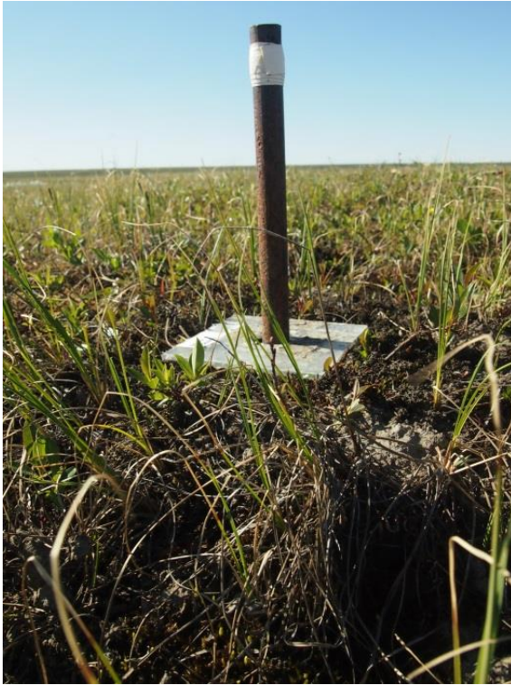
Figure 2. a) Metal pipe, anchored in permafrost; b) fiberglass rod, anchored in permafrost.
