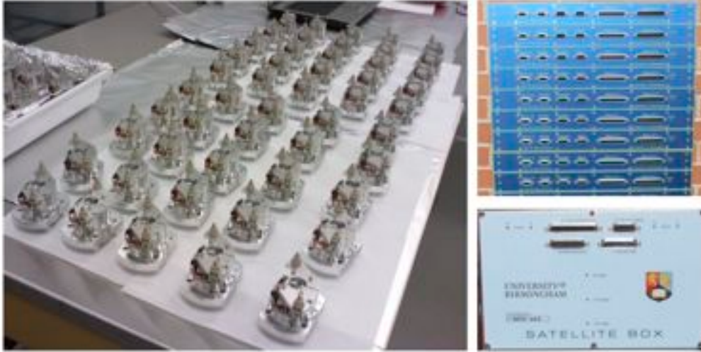
Figure 12. Pictures of the final production articles. On the left, BOSEM units during assembly and inspection in the clean room facilities. Top right: a stack of PUM coil-driver units. Bottom right: the front panel of a satellite box.
