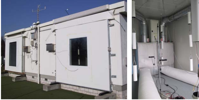
Fig. 1 Outdoor view (left) of test cells with two removable façade elements (3.4 m × 3.4 m) and indoor view (right) showing HVAC cabinet and extract and supply ducts.
