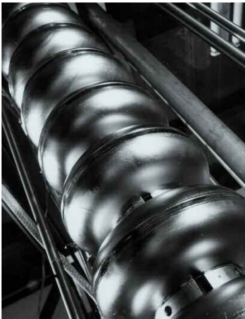
Superconducting accelerator structures made of niobium, developed for research towards a future linear collider.
