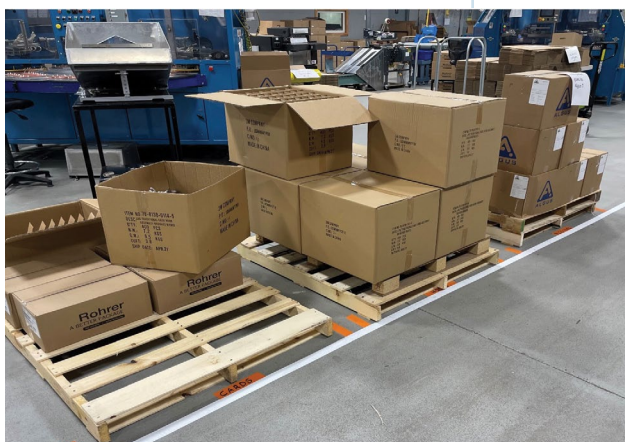
To improve organization, pallet locations are now marked for correct placement, reducing lost time locating raw materials.
