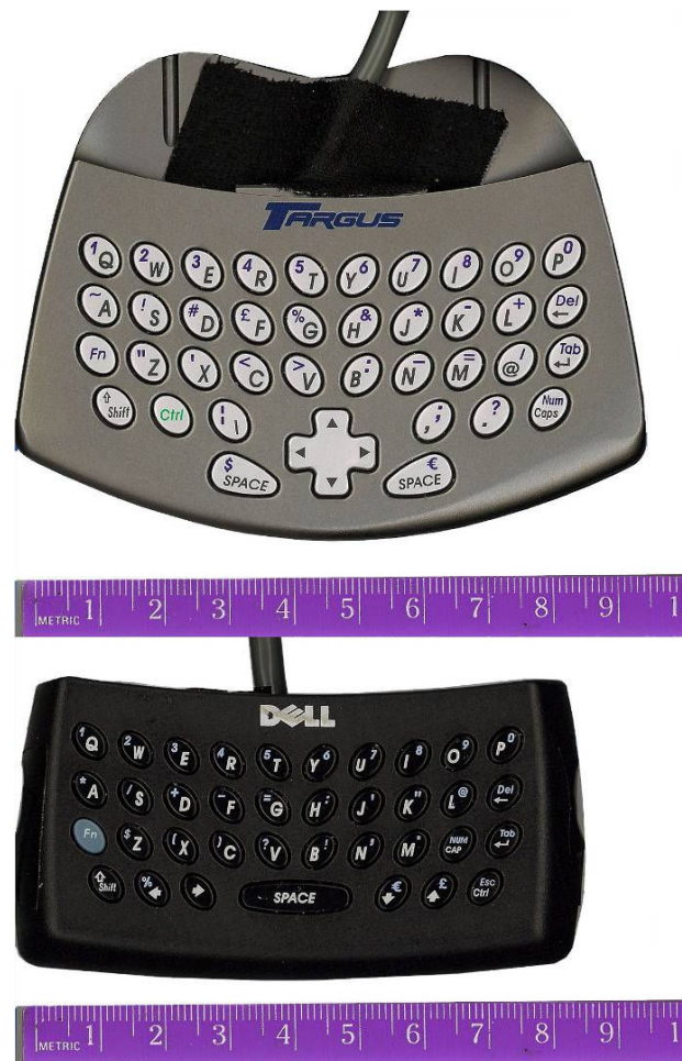
Figure 2. The modified Targus (top) and Dell (bottom) keyboards.
