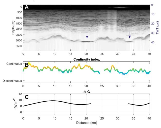
Example of radargram, continuity index and  $\Delta G$  values for a radar line. If the value for  $\Delta G$  is below  $5 \text{mW/m}^2$  it is not shown in the plot.
