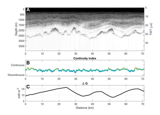
Example of radargram and continuity index for a radar line (here  $\Delta G$  is below threshold value).
