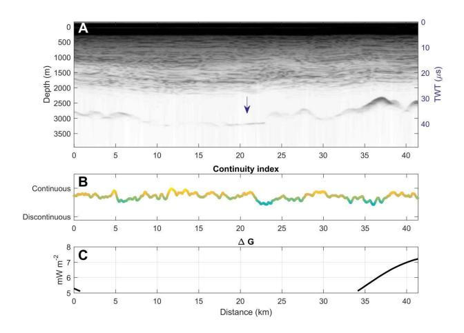
Example of radargram, continuity index and  $\Delta G$  values for a radar line. If the value for  $\Delta G$  is below 5mW/m<sup>2</sup> it is not shown in the plot.
