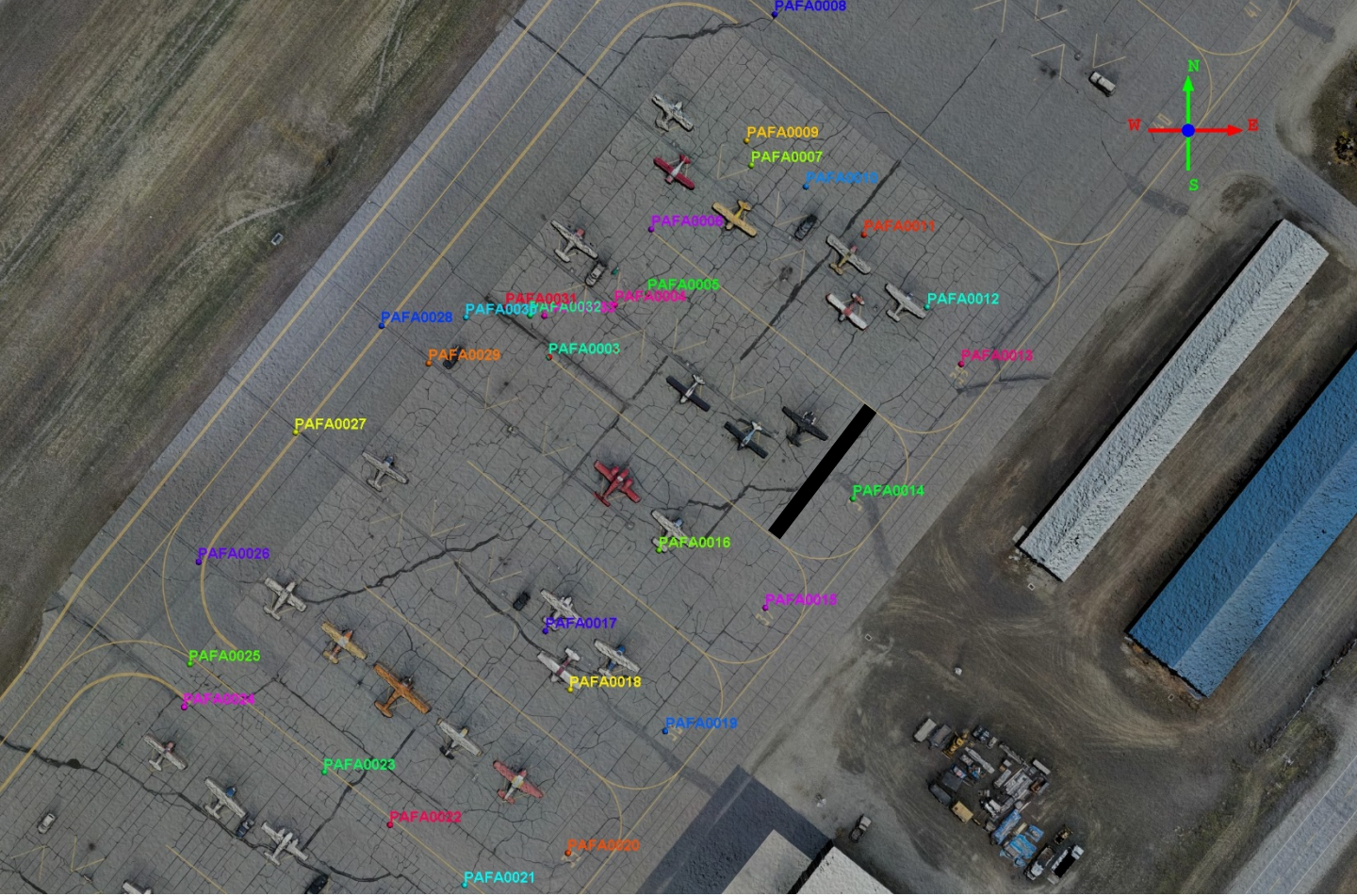
Figure S2 A-B. GCPs from Fairbanks International Airport. These photo-identifiable GCPs were made on taxiway letters and intersections of lines or cracks. Black scale bar shown in each photo is approximately 33 m long.
