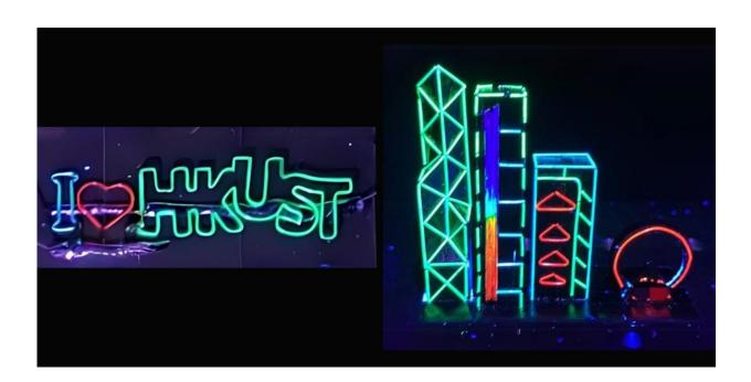
Photoluminescence of flexible full-color Fi-LEDs: I ♥ HKUST pattern (left) and "night scene" of Victoria Harbor showing color transition (right), built by mounting batches of fibers. Credit: HKUST
