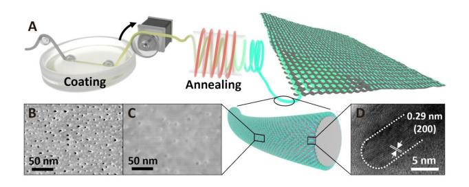
The growth of perovskite quantum wires with porous alumina membrane template. Credit: HKUST
