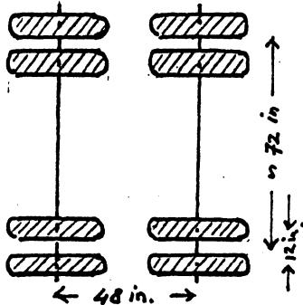
The 40 Kip load is applied over 8 tires. Thus, each tire bears 5000 Lbs (22.2 kN) load with 100 Psi (690 kPa) tire pressure. The contact area of each tire,  $A_c$  = Load of each tire/tire pressure =  $5000/100 = 50 \text{ in.}^2 (8.2 \times 10^4 \text{ mm}^2)$ . The dimension of the contact area is :
