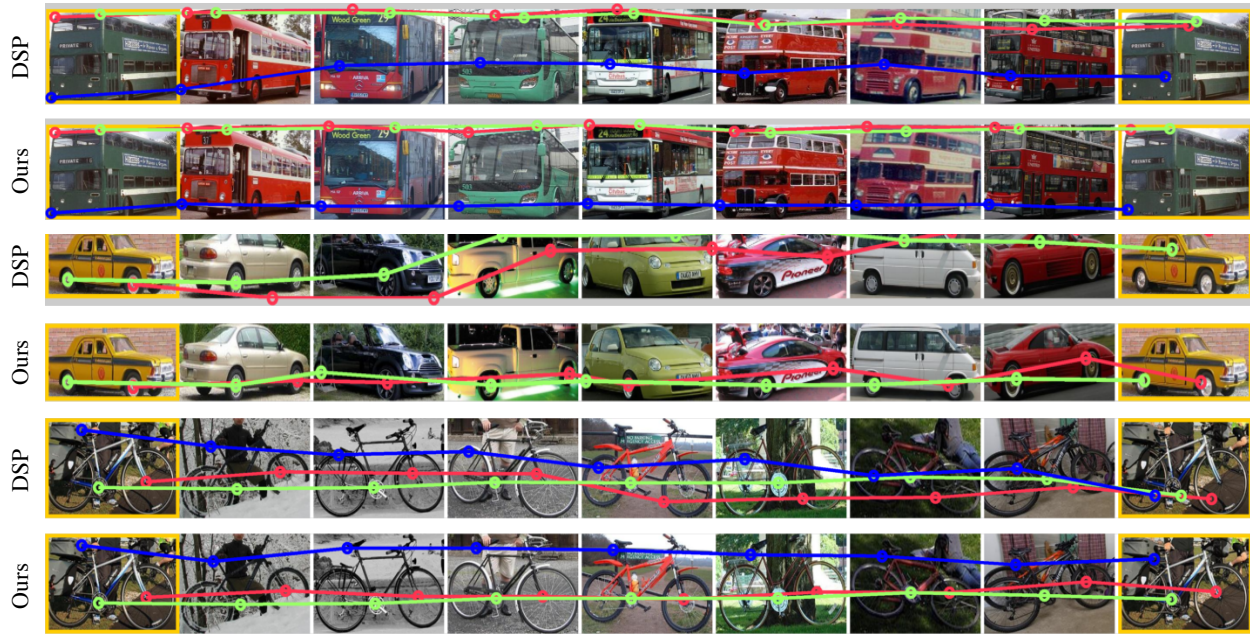
Figure 5. Comparison of keypoint correspondence tracks along a cycle in the graph (the first and the last image is the same for all examples) between DSP (initialization to our method) and ours. The keypoint correspondences become much more accurate and cycle-consistent after our joint alignment procedure.
