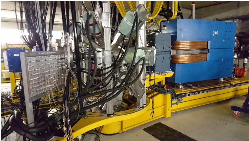
Figure 3: The K600 magnetic spectrometer with the Clover detectors from AFRODITE and large-volume LaBr 3 :Ce detectors.
