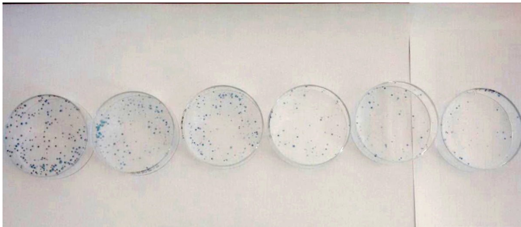
Figure 1: Cell survival of samples irradiated to the same dose at 6 different positions in the distal edge of the proton therapy beam. A large variation of radiation quality is evident.
