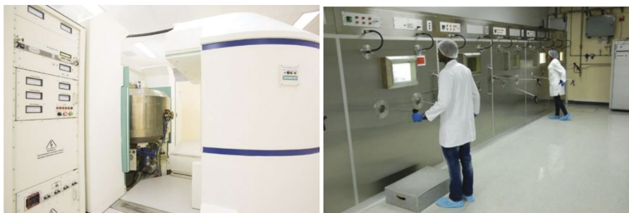
Figure 3. 11 MeV cyclotron dedicated to ^{18}\text{F} production (left) and hot cells for chemical processing of radio-pharmaceutical isotopes produced with high-intensity 66 MeV protons from the SSC (right).
