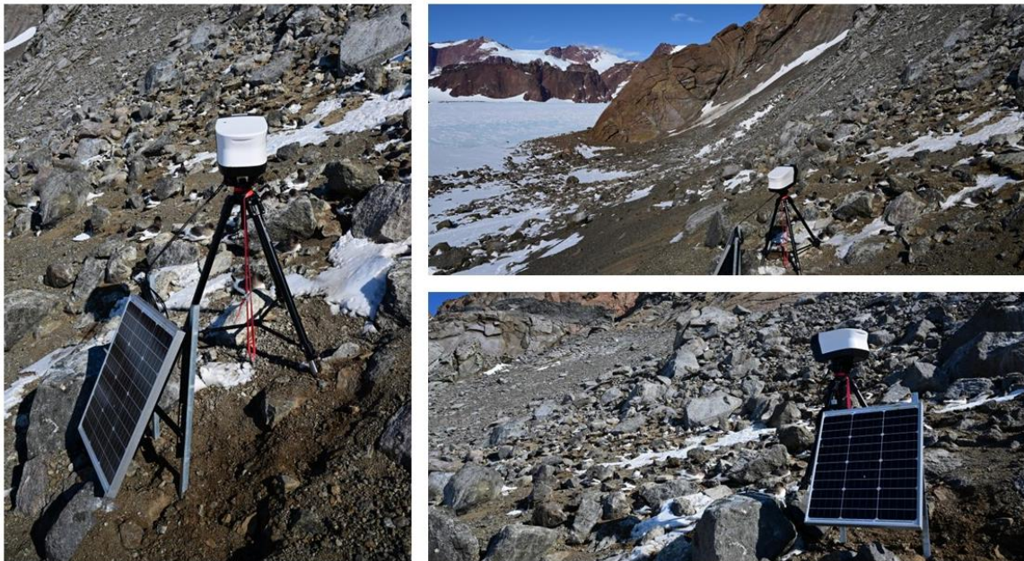
The camera systems in Jutulsessen after the upgrade in summer 2023/24. Photos: Sebastien Descamps, NPI.
